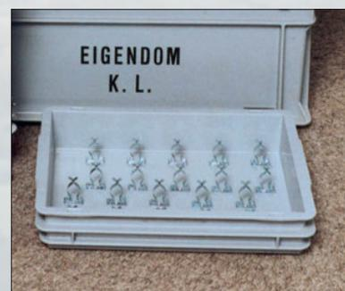
Clips will take a spare set of 12 injectors for a Leopard Tank (Multifuel solution).
